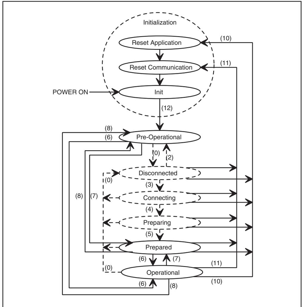
The KEB-CANopen-interface connection realizes following transitions, illustrated in the above diagram by a solid line:
