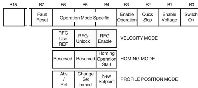
The Bits B6 to B4 are defined mode-dependent. Grey highlighted Bits are currently not realized in the KEB-CANopen-interface connection.
