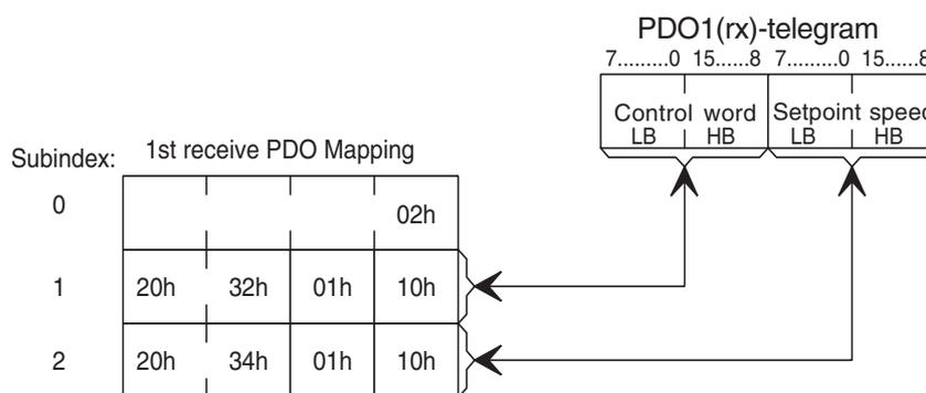
*Example for the coding the data on the CAN-BUS:*
