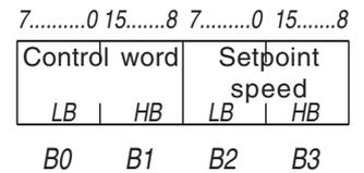
The length and assignment of the PDO2(rx)-telegram can be changed by different operator-parameters . This change can be made only by the SDO(tx)-telegram (see above).
