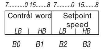
The length and assignment of the PDO1(rx)-telegram can be changed by different operator-parameters. This change can be made only by the SDO(tx)-telegram (see above).
